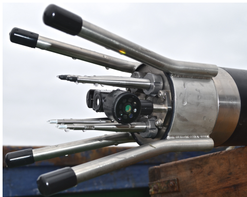
Figure 5. Sensor head of Rockland Scientific VMP-250
