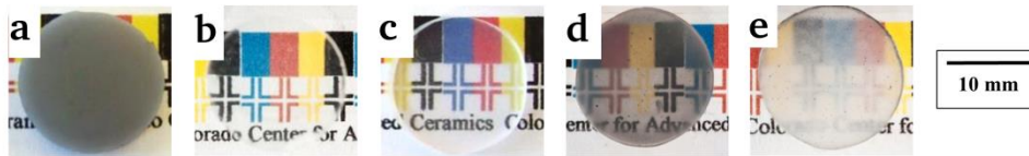
Fig. 4.13: Compacts hot-pressed using the standard profile with (a) sulfate powder, (b) sulfate powder with 1 wt% LiF, (c) sulfate powder with 1 wt% LiF but with pressure applied at 900°C, (d) alkoxide powder and (e) alkoxide powder with 0.25 wt% LiF (compacts 10 mm above template).
