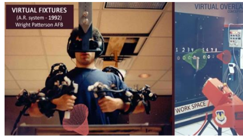
Figure 1 The first AR system with virtual fixtures at U. S. Air Force's Armstrong Laboratory [8]
