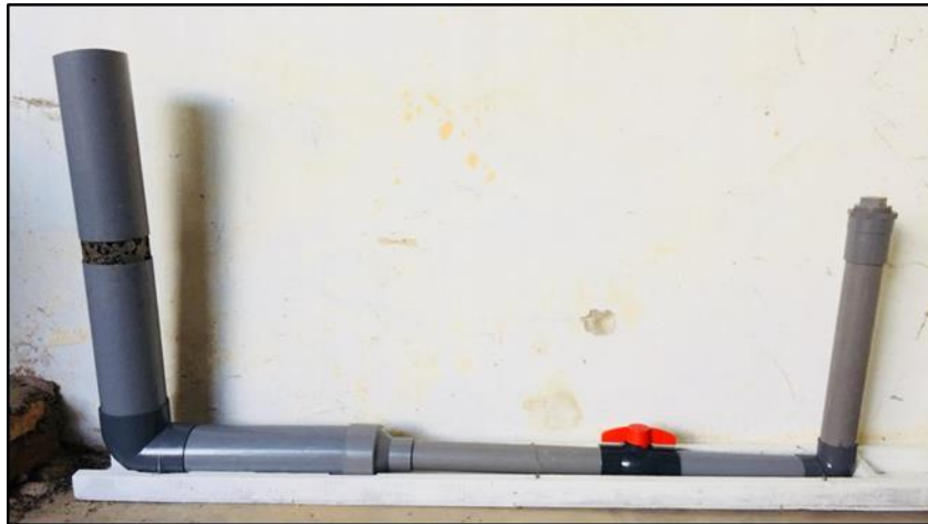
Figure 3. Permeability Test Instrument
