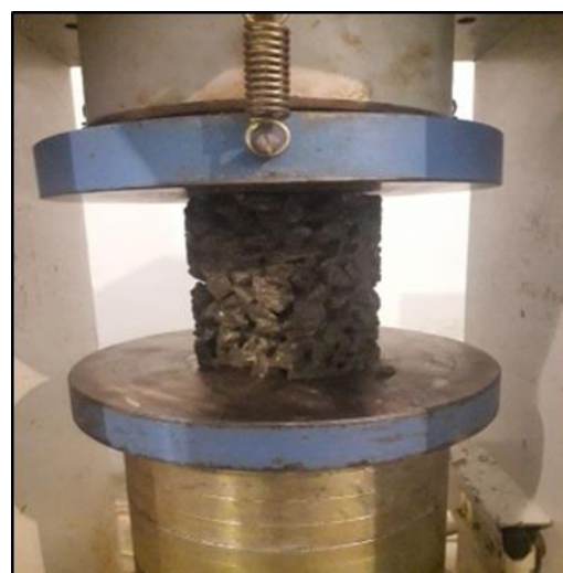
Figure 2. Compressive Strength Test
