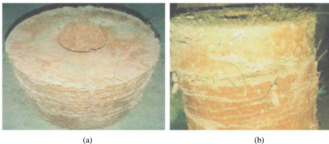
Figure 2. Clay-Coir Fiber Samples for CBR Test, (a) top view of soil specimen for CBR test (b) soil specimen with coir fiber mixing stabilization
