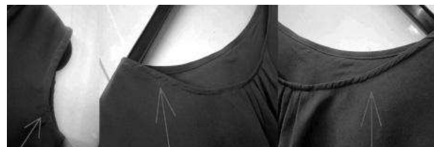
Figure 2: Seam puckering in armhole (left) and neckline (central and right), fabric F1
