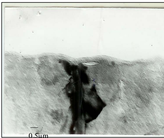
Fig.1 Transmission Electron Micrograph of the coating developed for 5mins in non-chromate bath.
