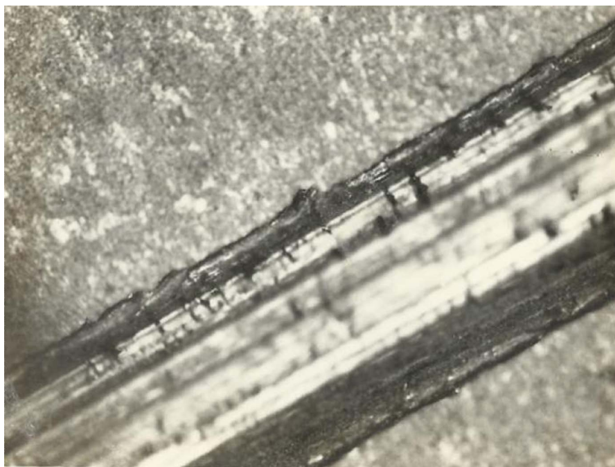
Figure 1. Optical photograph of a conversion coated aluminium with a top coating of lacquer after exposure to high humidity for 255 hours without paint delamination at the edge of a pre = scratched region and no pitting corrosion. \times 1000 .
