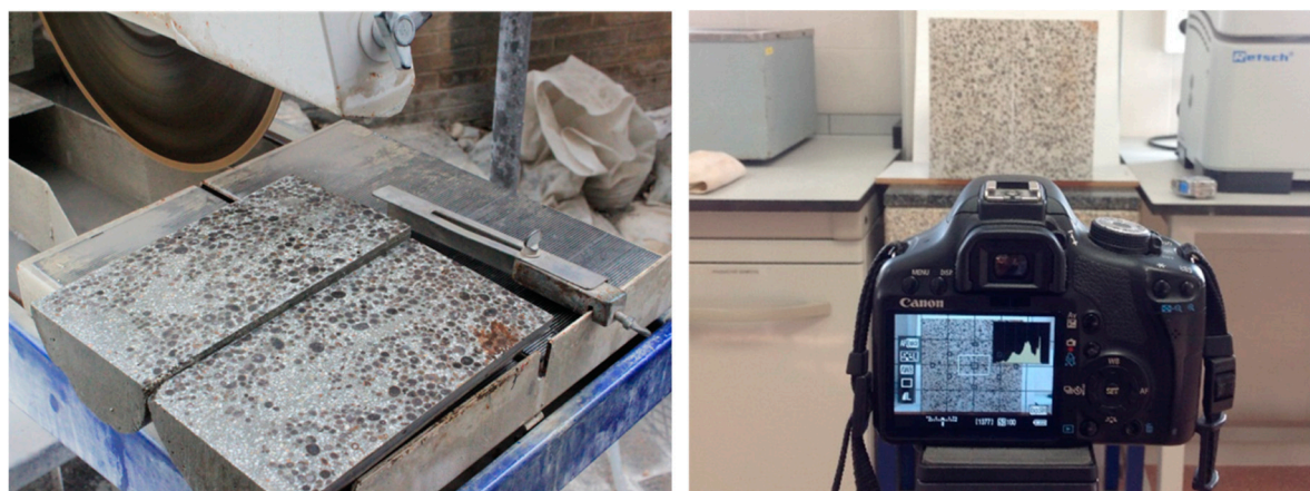
Figure 2. Left: saw cutting of the specimens into halves. Right: photographing of the halves.
