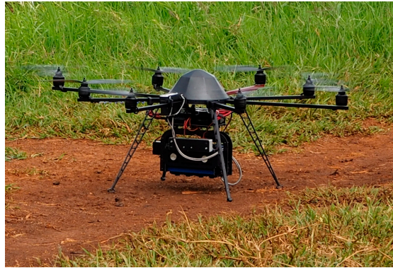
Figure 3. Mikrokopter OktoXL 6S12 unmanned aerial platform equipped with the micro-MCA12 Tetracam multispectral sensor, showing the placement of the Incident Light Sensor (ILS) module with white diffuser plate connected by a fiber optic cable to the top of the UAV facing upwards while the other 11 multispectral sensors are positioned on a dual axis gimbal camera platform for zenithal/nadir image capture. The RGB (Red-Green-Blue) and TIR (thermal infrared) cameras were alternately mounted on the same gimbaled platform for image capture.
