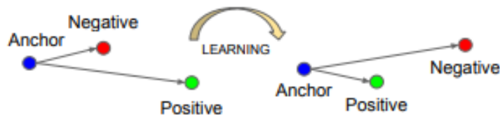
Figure 4.1: Triplet loss minimizing the distance between the anchor and the positive as well as maximizing the distance between the anchor and the negative. Image font: Cornell University
