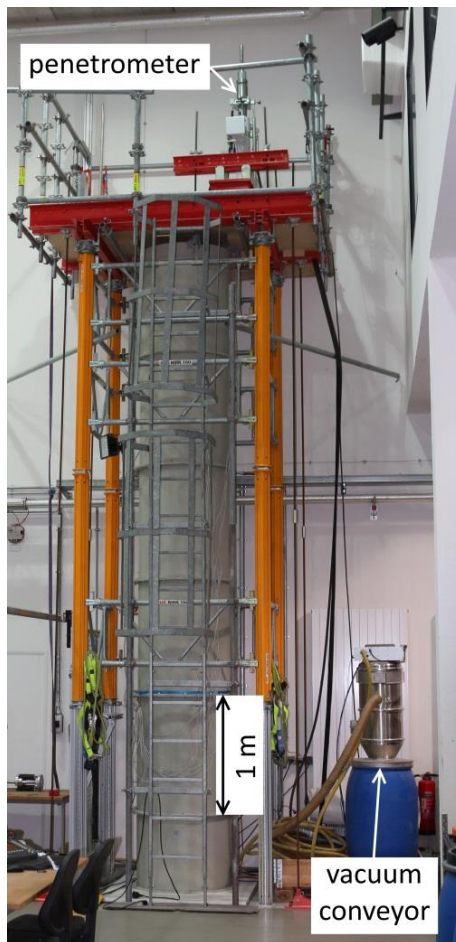
Figure 7: Deep penetration testbed (left) with penetrometer (top) and vacuum conveyor (bottom right)
