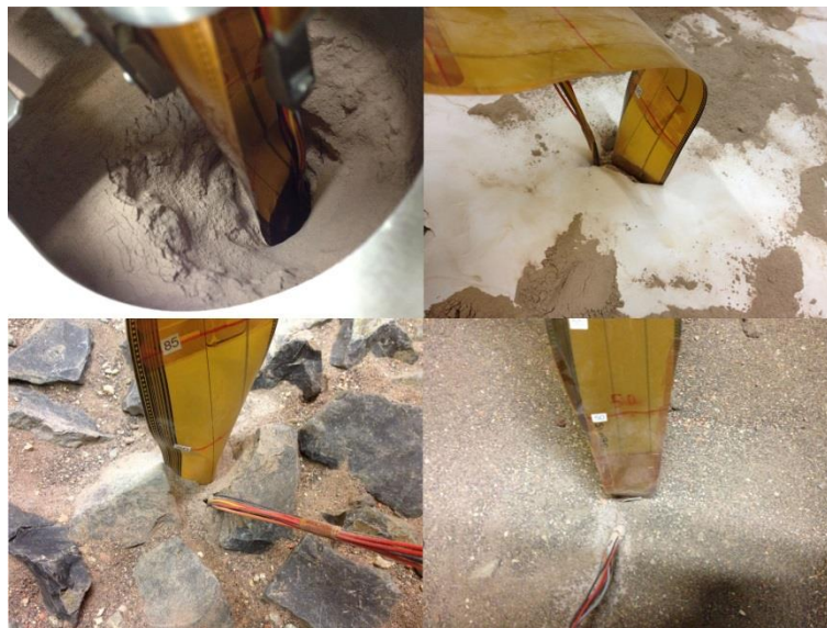
Figure 20: Different layers for the layers test: MMS dust (top left), paper (top right), rocks (bottom left) and MMS sand (bottom right)
