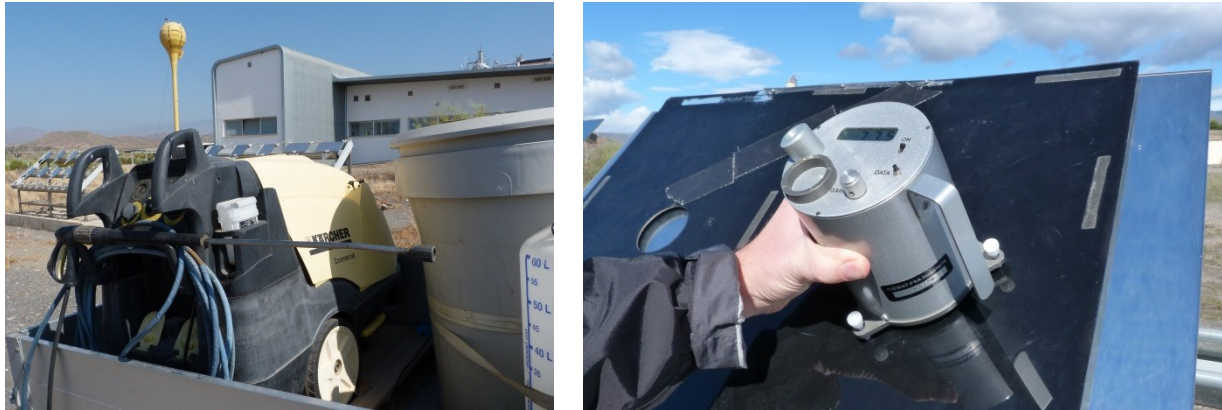
135 Figure 2: a) Kärcher cleaning device and b) D&S reflectometer placed on measurement mask.
