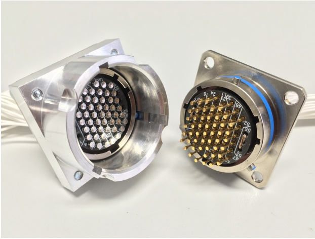
Fig. 10 MASCOT Umbilical Connector (UMC) comprising of two identical MIL standard matrix KJ type bodies equipped with spring-loaded pogo pins on one side and concave counter pins on the other
