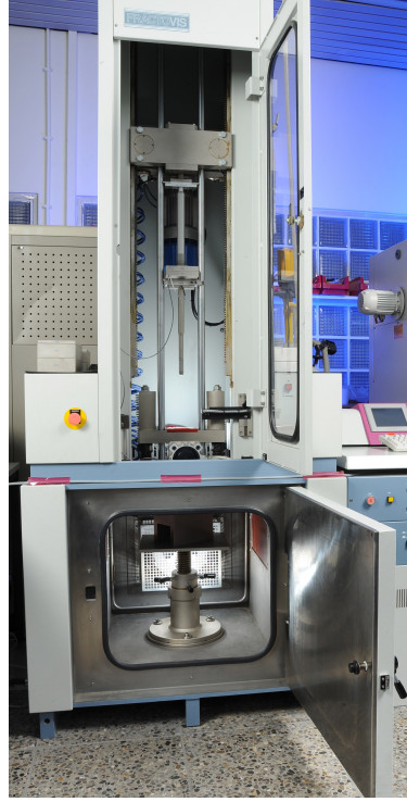
FIGURE A.1: Ceast Fractovis impact drop tower that was used to conduct the experiments for this work.
