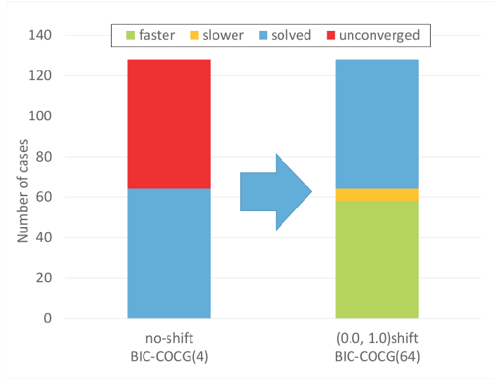
Fig. 2: Effect of the regularized IC preconditioner with the COCG method. By using the diagonal shifted block IC-COCC (BIC-COCC), we can solve all test problems from our benchmark set.
