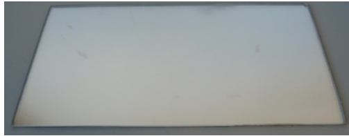
FIGURE 1. Picture of one of the reflector samples with anti-soiling coating, manufactured by Tekniker and Rioglass
