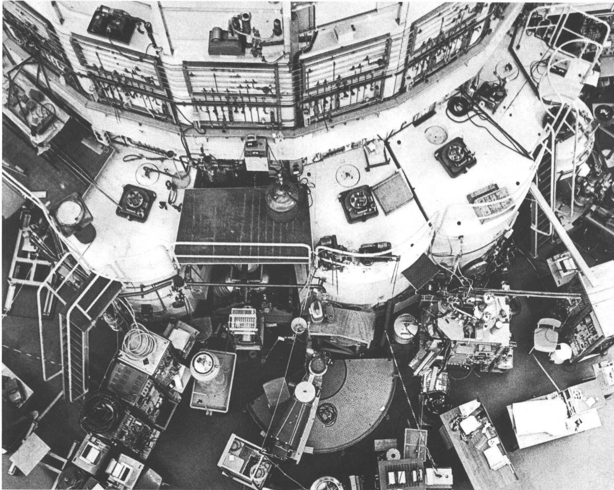
HFR ground-floor. Some experimental set-ups for basic research using the horizontal beam tubes.
