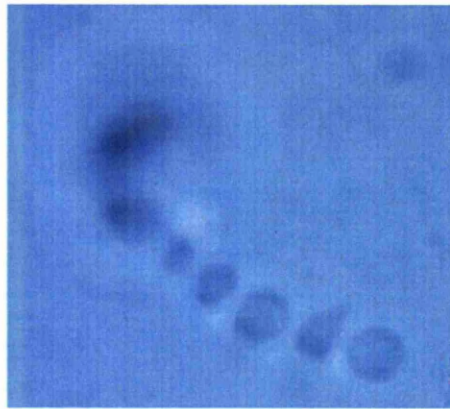
Figure 2.8: Showing the produced ‘tethered tool’. The darker top left corner of the tool is fixed to the surface. The rest of the tool can be manipulated using several optical traps using SLM. Taken from (44).
