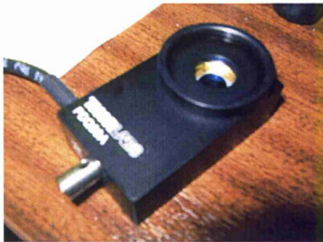
Figure 3.20: Image of the Quadrant detector device (left). Setup of the four quadrants for measuring beam position (right).
