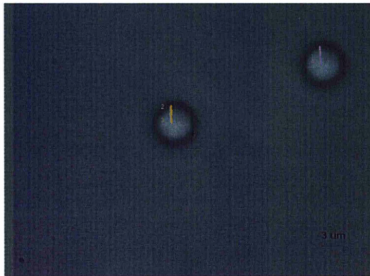
Figure 4.2: Plot produced from StAT. The centre sphere is optically trapped. The sphere to the right is fixed to the surface the, and hence its movement is equivalent to that of the stage. The pink and yellow lines show the movement of the spheres as tracked by the StAT program.
