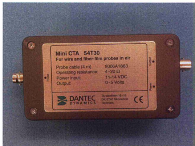
Figure C.11: Dantec Dynamics mini constant temperature anemometer.
