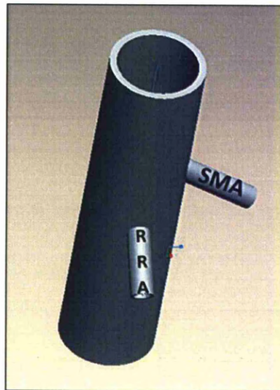
Figure 4.1 A 3D computer-aided design (CAD) image of the aortic neck phantom used in the validation of the CT CLL migration measurement technique
