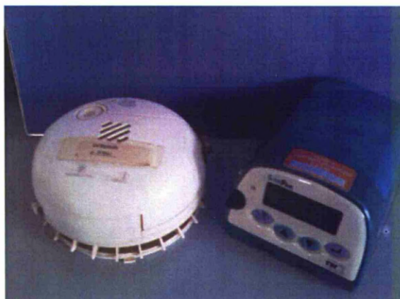
Photometric analysis – A University of California, Berkeley sampler and a TSI Sidepak.
