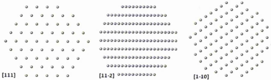
Figure 7.34 ATOMS ® model of iron perfect crystal in different orientations. This confirmed no irregularity in the crystal.
