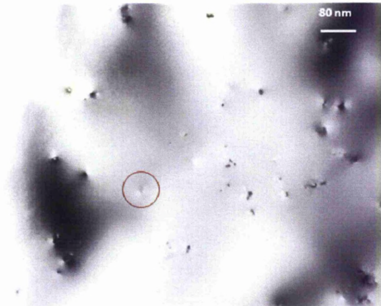
Fig.8.37. TEM bright field image of screw dislocations in [111] direction recorded at 20kX magnification. Screw dislocation shown in the red circle is visible with a faint contrast. The dislocations that are visible in the TEM are recorded and the location of them is mapped using low magnification images. The single crystal samples were much cleaner than the polycrystalline samples without oxides or deposits on the surface. This made the identification of screw dislocations much easier in the TEM.
