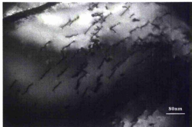
Figure 5.5 Bright field TEM micrograph showing dislocations inclined to the surface of the foil.
