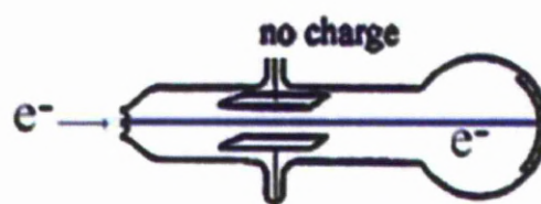
Figure 2.1: Flow of electrons when no electric field was applied
