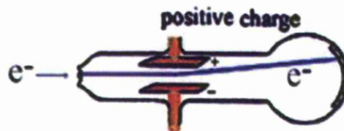
Figure 2.2: Electron deflection once the electric field was turned on
