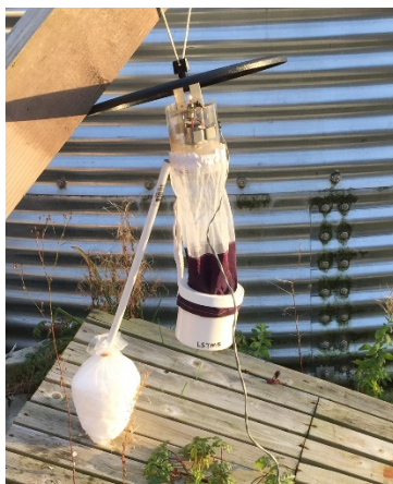
Figure 4.2: A CDC light trap with dry ice to provide CO 2 .
