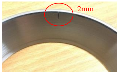
Figure 3. Bearings with seeded defects on the outer race
