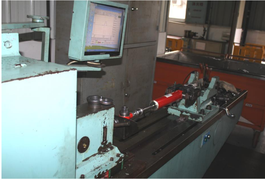
Fig. 5 Bench testing of a high-speed rail pantograph hydraulic damper
