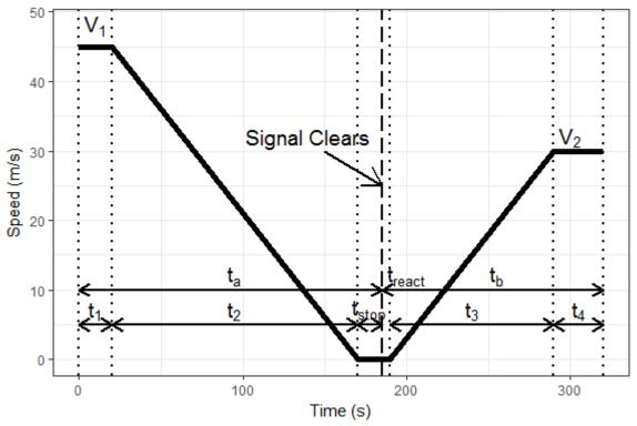
Figure 2 Example Speed Profile for CSS Signal Approach
