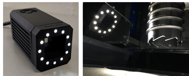
Figure 5: The SurfCam prototype integrated into the LUVMI rover NavCam
