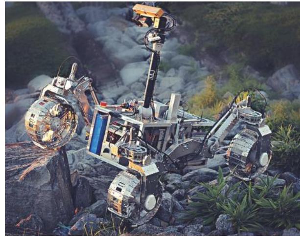
Figure 2: LUVMI rover, highlighting obstacle clearance
