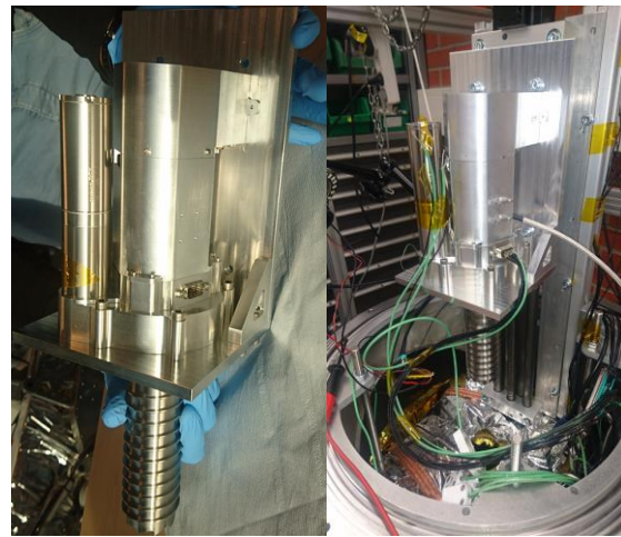
Figure 10: (Left) The integrated VS & VA instruments (Right) The VS & VA mounted in the environmental chamber at TUM prior to end-to-end testing with lunar simulant material
