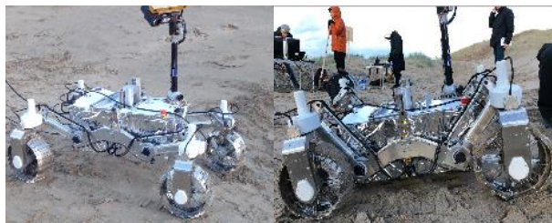
Figure 1: Left - nominal chassis height for navigation. Right: lowered chassis to perform drilling operation.
