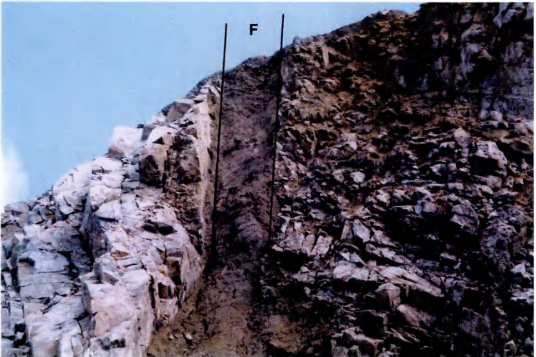
Figure 3.4a. (Upper photograph). Vertical fault or joint planes approximately 650 mm wide, filled with pale-grey material from the Central Quarries of the Penmaenmawr Intrusion.
