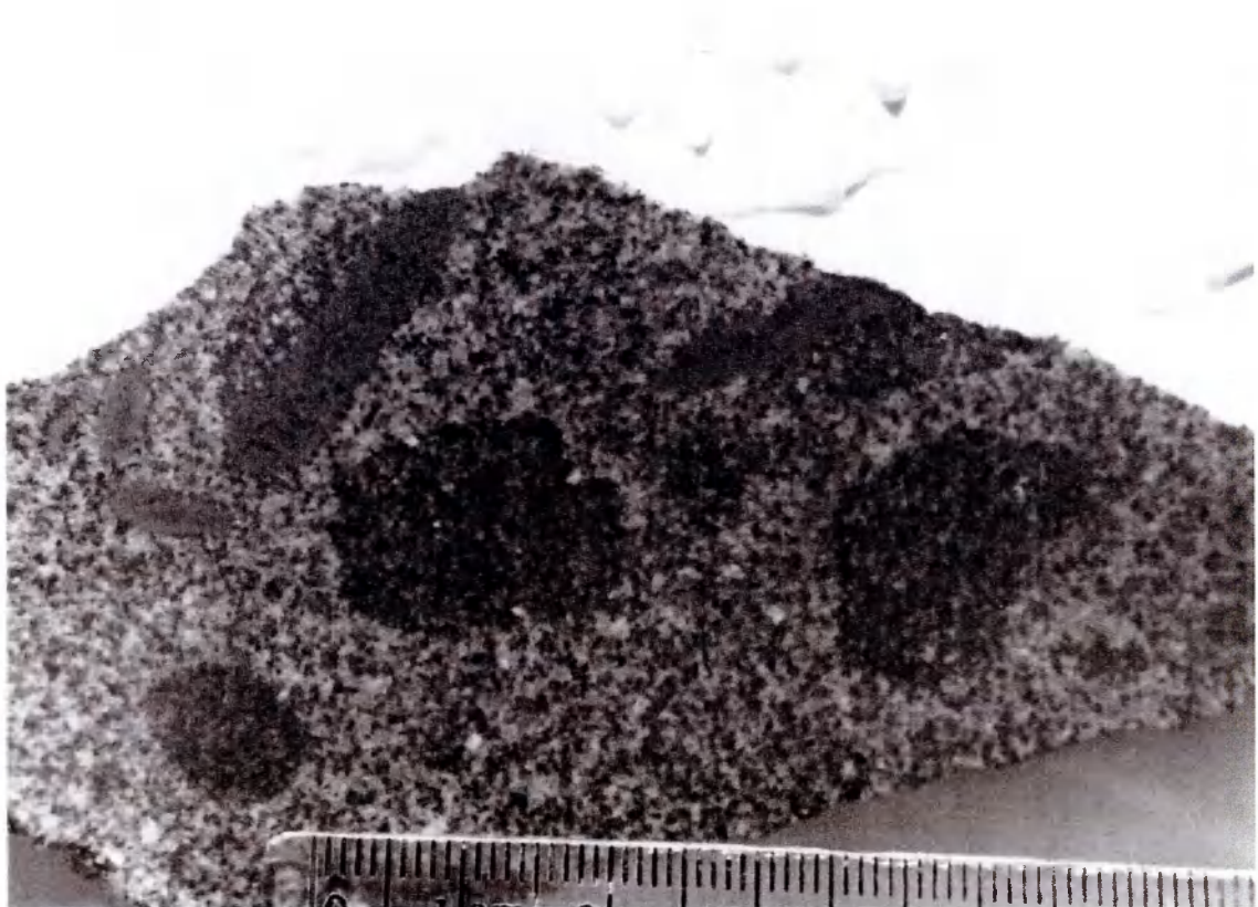
Figure 3.2. (Upper photograph). An irregular segregation from the Central Quarries of the Penmaenmawr Intrusion.
