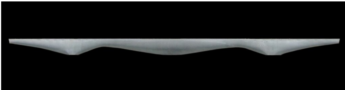
Figure 8 Fabric-cast concrete 'bending moment' beam (courtesy of Mark West)
