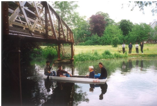
Figure 4 Concrete punt (Tim Ibell at front)
