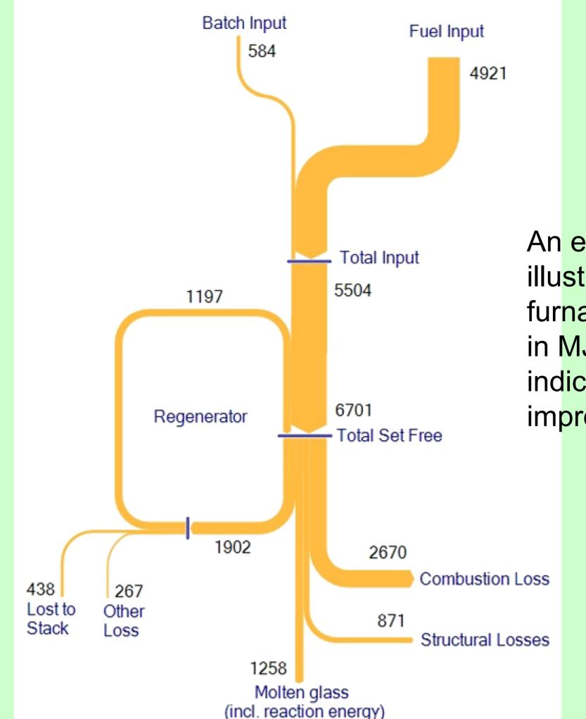
An exergy analysis, such as that illustrated here, for a glass furnace, showing flows of exergy in MJ per tonne of output, can indicate areas of a process where improvement is possible.
