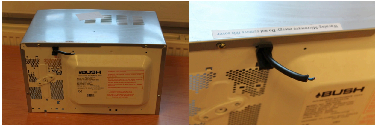
Picture 7: Microwave with fixed cable (broken).
