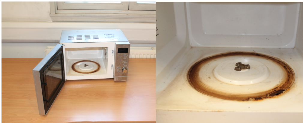
Picture 5: Microwave oven with rusted internal cavity.
