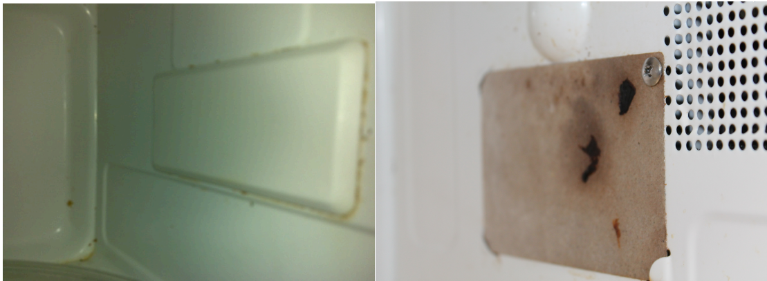
Picture 6: Plastic and mica wave-guide cover
