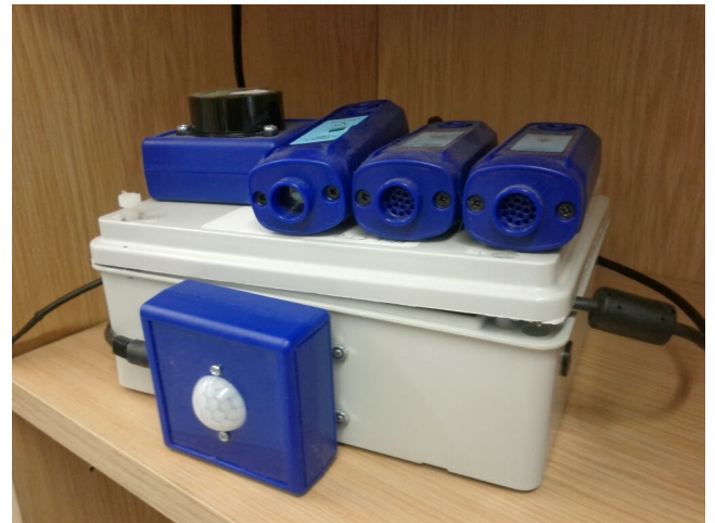
Figure 1: Sensor box in situ ., showing PIR, temperature, CO 2 , light, sound and humidity sensors.
