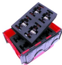
Fig. 1.1. Soft material packaging example for mass produced parts
