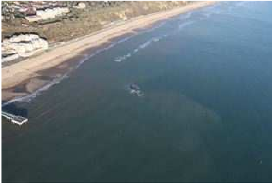
Figure 10. Aerial view of the beach response in the lee of Boscombe Reef (10 March 2010)
