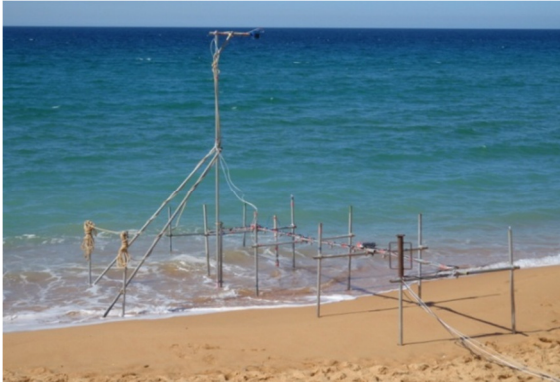
Figure 3 Photograph showing the field instrumentation deployed on a scaffolding rig. The rig was deployed just above MSL at high tide to ensure that swash excursions occurred within the LiDAR field of view.
