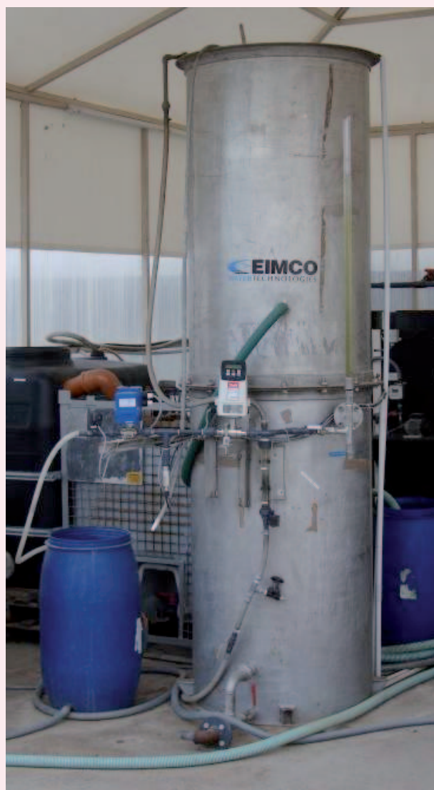
Figure 2: Photo of the pilot MBR installation
