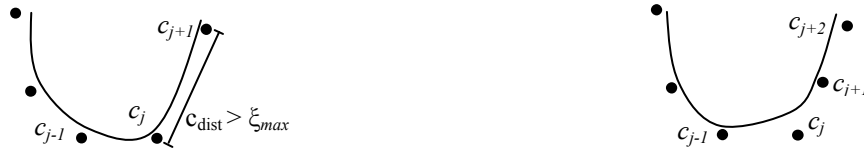
(a) B-spline before a control point has been inserted (b) B-spline after a control point has been inserted
