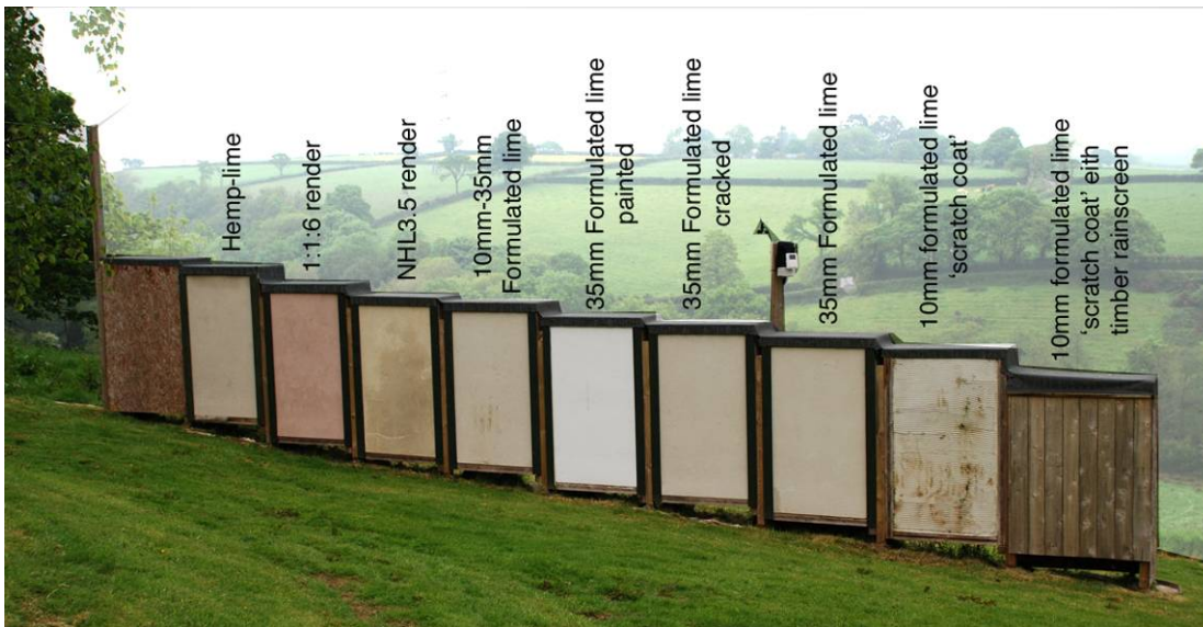
Figure 3: Sample panels on exposure site in South Cornwall
