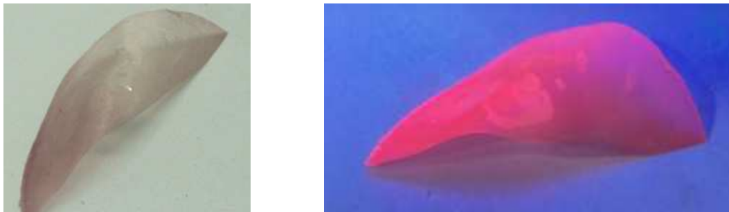
Figure 1 (a) (b) Fluorescent nanocomposite film observed under visible light (a) and under ultraviolet light at the wavelength of 365 nm (b)
