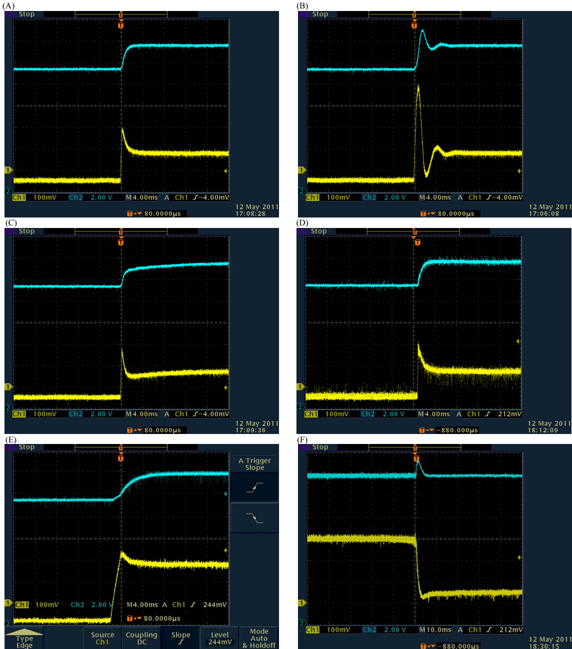
Fig. 6. Step response 12 – 14 V: a) Optimal filter cut off frequency = \omega_{opt} . b) Filter cut off frequency = 2 \omega_{opt} . c) Filter cut off frequency = \omega_{opt} / 2 . d) Input voltage V_g = 100 Vdc. e) Input voltage V_g = 5 Vdc f) Step load resistance change 0.3\Omega to 1\Omega V_o = 14 Vdc. (Yellow trace = Output Voltage 2 V / division. Cyan trace = Inductor current 2 A / division).
