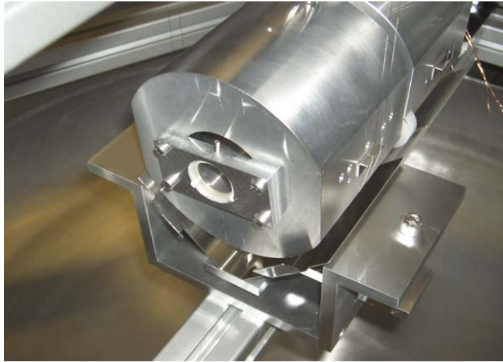
Figure 4.8 — Picture of the suspended grating. The 1" substrate was mounted on a jig which was in turn attached to the aluminum test mass.
