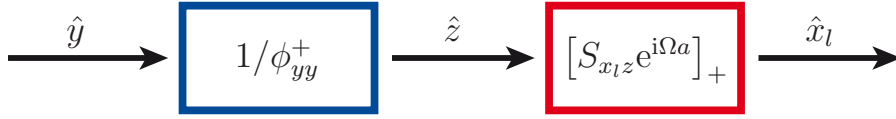
Figure 5.5.: Cascaded filtering process: output observable \hat{y} is transformed into a white noise process \hat{z} without loss of information. Then the Wiener filter is applied to \hat{z} in order to obtain an optimal estimate for \hat{x}_l .
