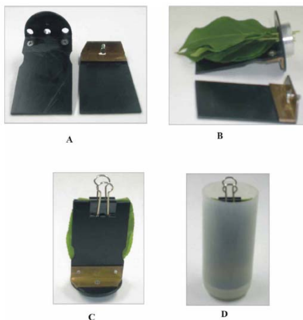
Fig. 12. Home-made holder for apoplastic fluid isolation from leaves; A, holder without plant leaves; B, holder with plant leaves before fixing; C, fixed plant leaves within the holder; D, holder with plant leaves, ready for centrifugation.
