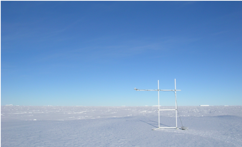
Figure 4.7: Photograph of albedo measurements performed at the ice edge. The SL501 is currently measuring incident radiation. The supporting frames of the equipment is painted white to minimise the shadowing effect.
