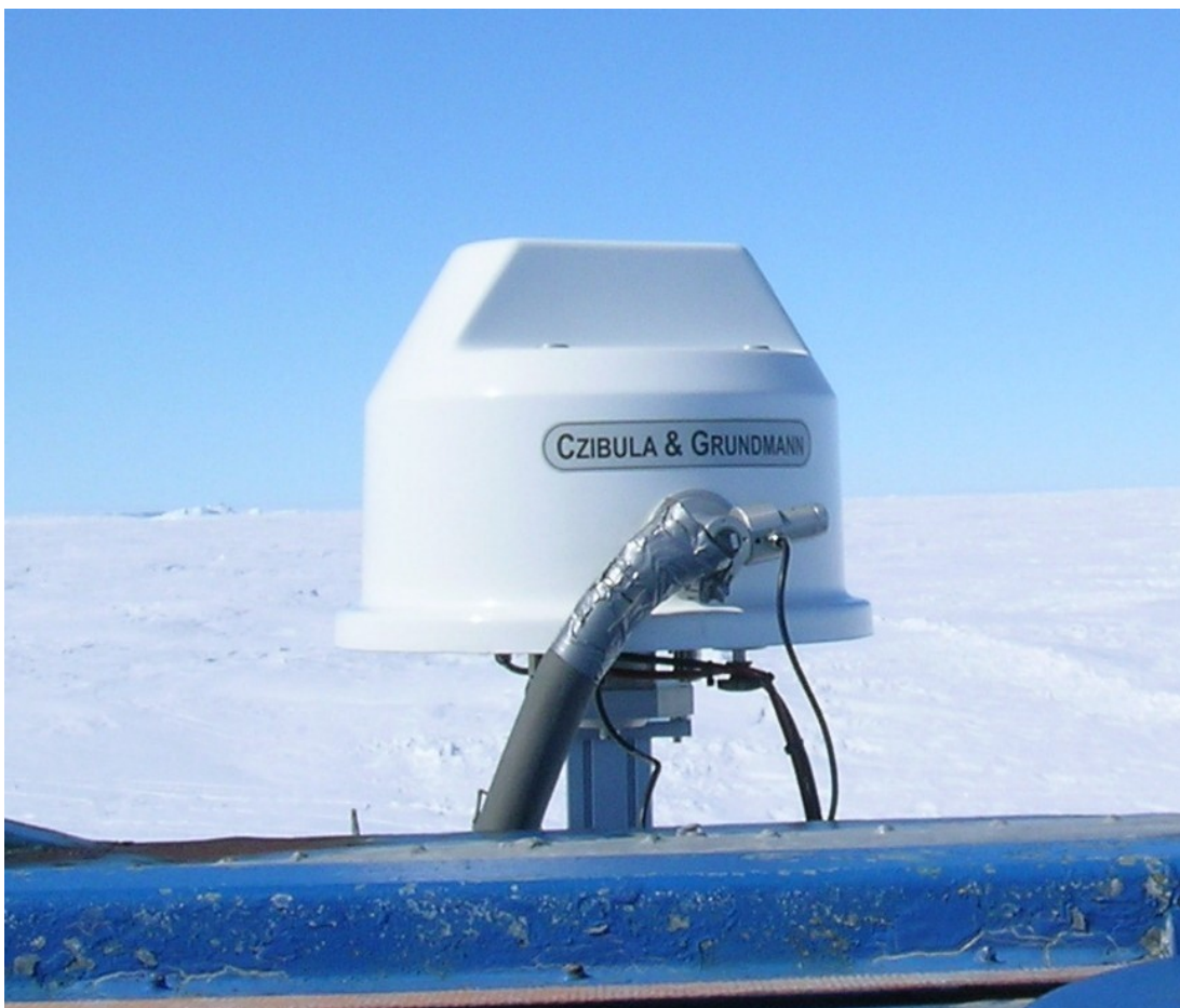
Figure 4.11: Skyscanner with the optical fibre attached for radiance measurements. Currently the entrance optics points near the horizon opposite the position of the sun. The optical fibre is protected by a flexible heated insulated tube.
