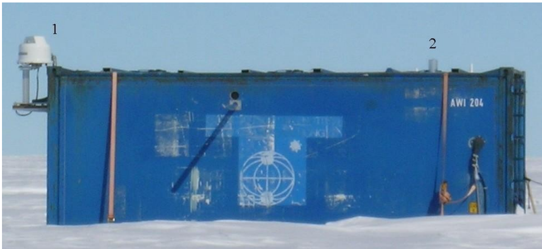
Figure 4.3: Container for radiation measurements during the summer campaign 2003/04. On the left, the Skyscanner (1) is mounted. The metal tube (2) on the right part of the roof holds the input optics for spectral irradiance measurements.
