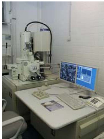
Fig. 6.5.2: Field-Emission SEM JEOL JSM-6700F.
