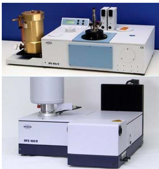
Fig. 6.5.3: IFS 66v/S Vacuum FT-IR spectrometer (top) and Bruker RFS100/S Raman spectrometer (bottom).
