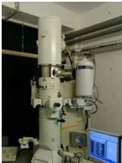
Fig. 6.5.1: JEOL JEM-2100F-UHR TEM microscope
