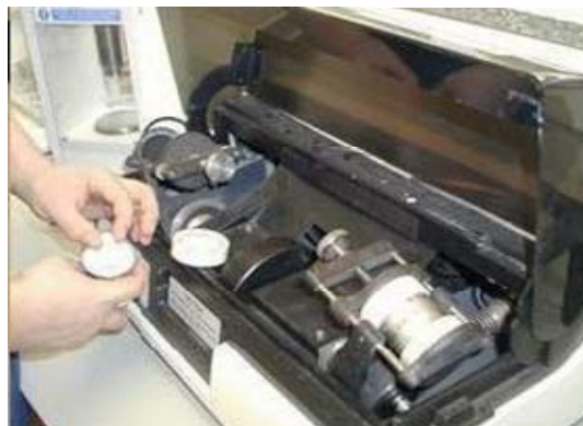
Fig. 5.1.1.: Loading of the SPEX 8000 mill.
