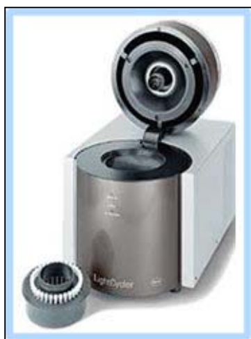
Figure 1.8.1 LightCycler (real time PCR equipment from Roche) used for the present study. (Illustration adopted from Lightcycler user manual, Roche).
