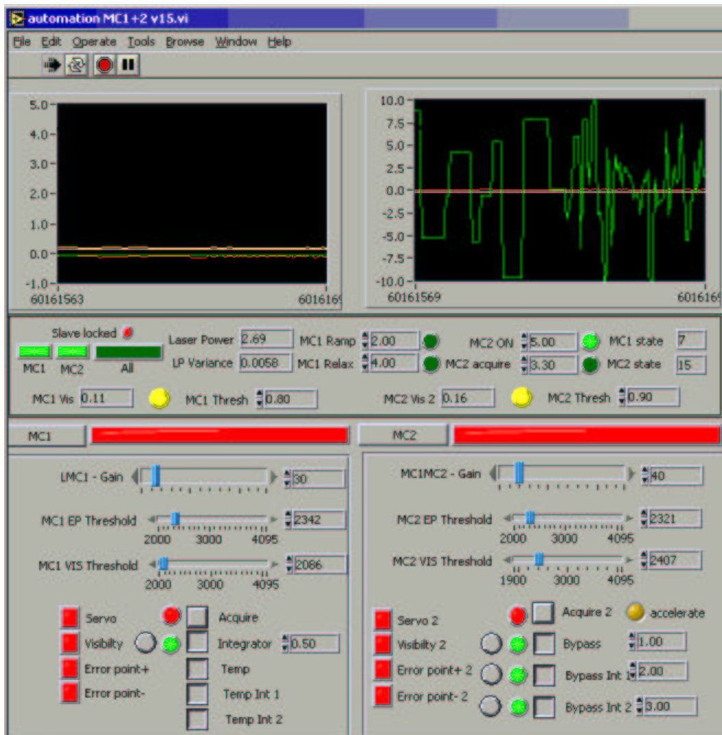
Figure H.2: Virtual instrument for supervising the control electronics for MC1 and MC2. The top left graph shows the visibility and error signals for both mode cleaners; the right graph shows the feedback signals. The center area contains various controls and indicators with respect to automatic operation. In particular, the green buttons (labeled ‘MC1’ and ‘MC2’) are used to switch the respective control loops to automatic operation. The lower part contains controls and indicators connected to the analogue loop filters: MC1 loop to the left and MC2 loop to the right.
