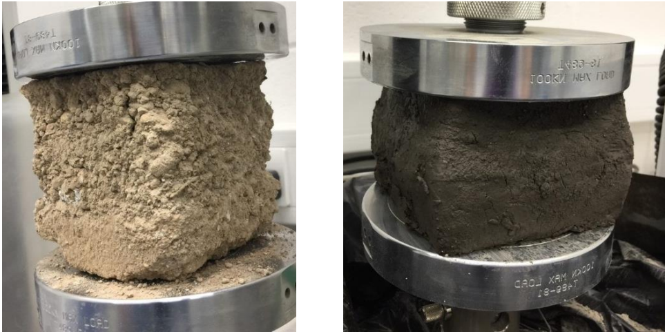
Figure 9: photographs showing a clay +10% lime sample on the left, and a natural clay sample on the right.
